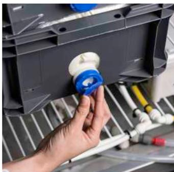
Remove each milk spigot and reseal the bladder connector using the milk suppliers seal. If this still leaks use the ½" bung supplied in your Parts Kit.
