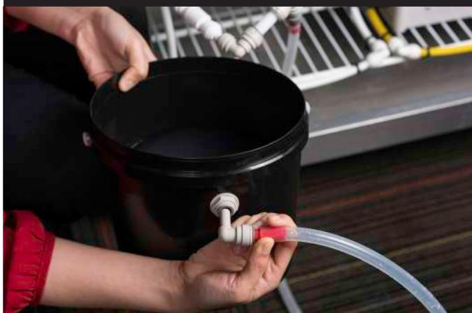
Fill the black cleaning bucket with cold tap water and connect the silicon cleaning line to the bucket.
