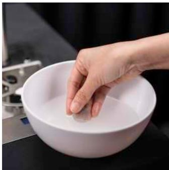
Gently clean each mesh filter in warm soapy water and then re-assemble in the order as shown in the picture, taking care to insert the large o-ring as the final piece of the assembly.
