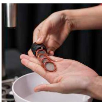
To disassemble gently push the filters and "O" Rings out of the filter housing into a large bowl so as not to lose any parts.
